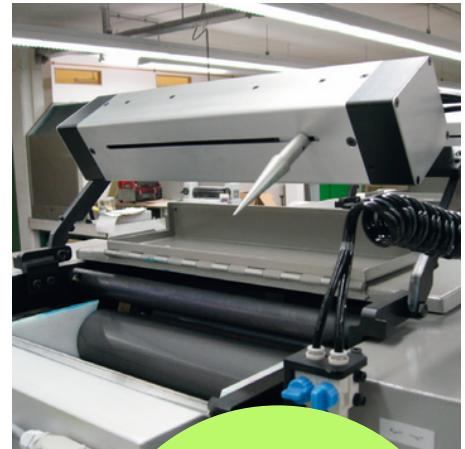
User friendly solution to avoid that the ink «stands still», especially with the use of high viscose UV-inks.
